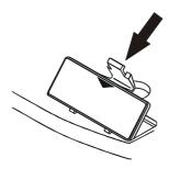
2.) Attach a fresh 9-Volt alkaline battery to the battery contacts as shown, and push the battery back into the battery compartment.
